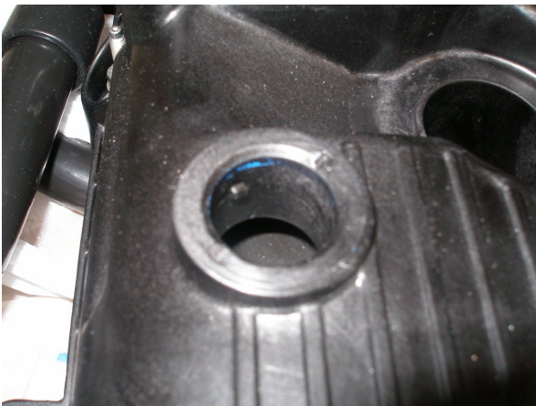
Rocker cover with nub for quarter-turn valve
